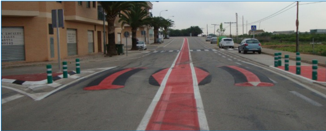
Figure 9: Speed Kidney - Image Source: FHWA
