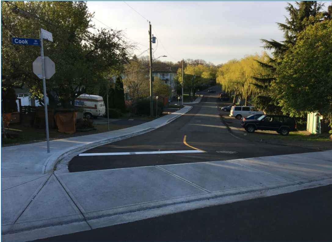
Figure 19: Sidewalk Extension - Image Source: City of Victoria
